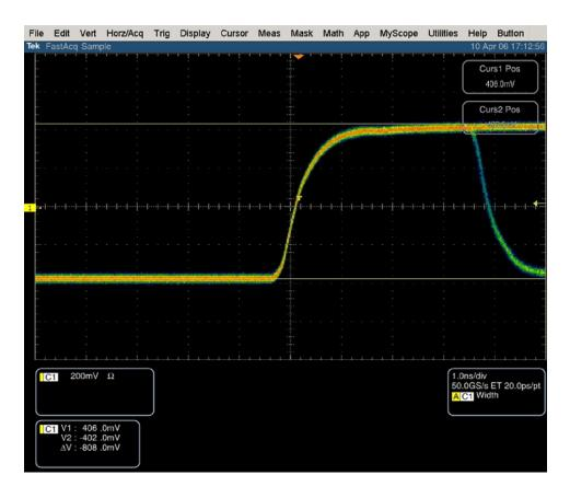
Figure 2-4: Trigger polarity negative
